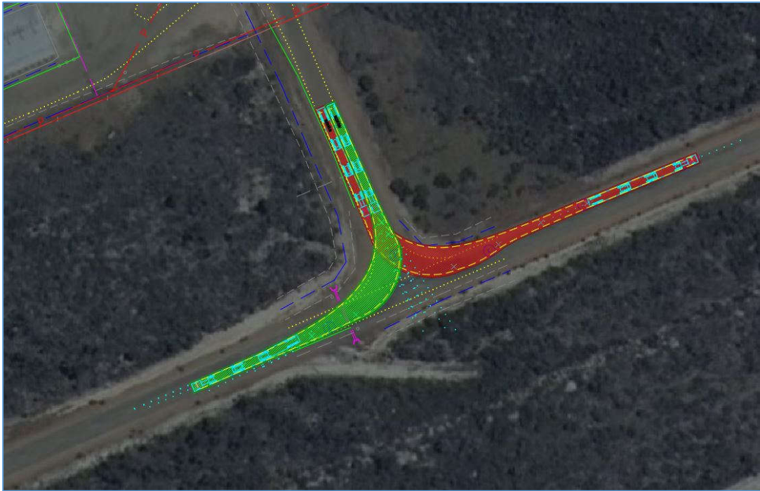
Figure 15: Exit Movement Swept Paths
