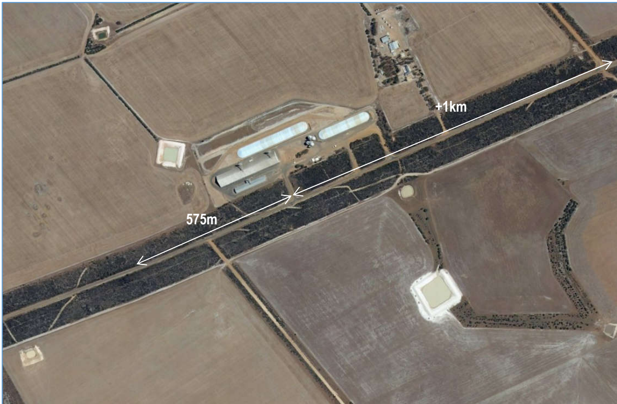
Figure 11: Site Exit Sight Distance
