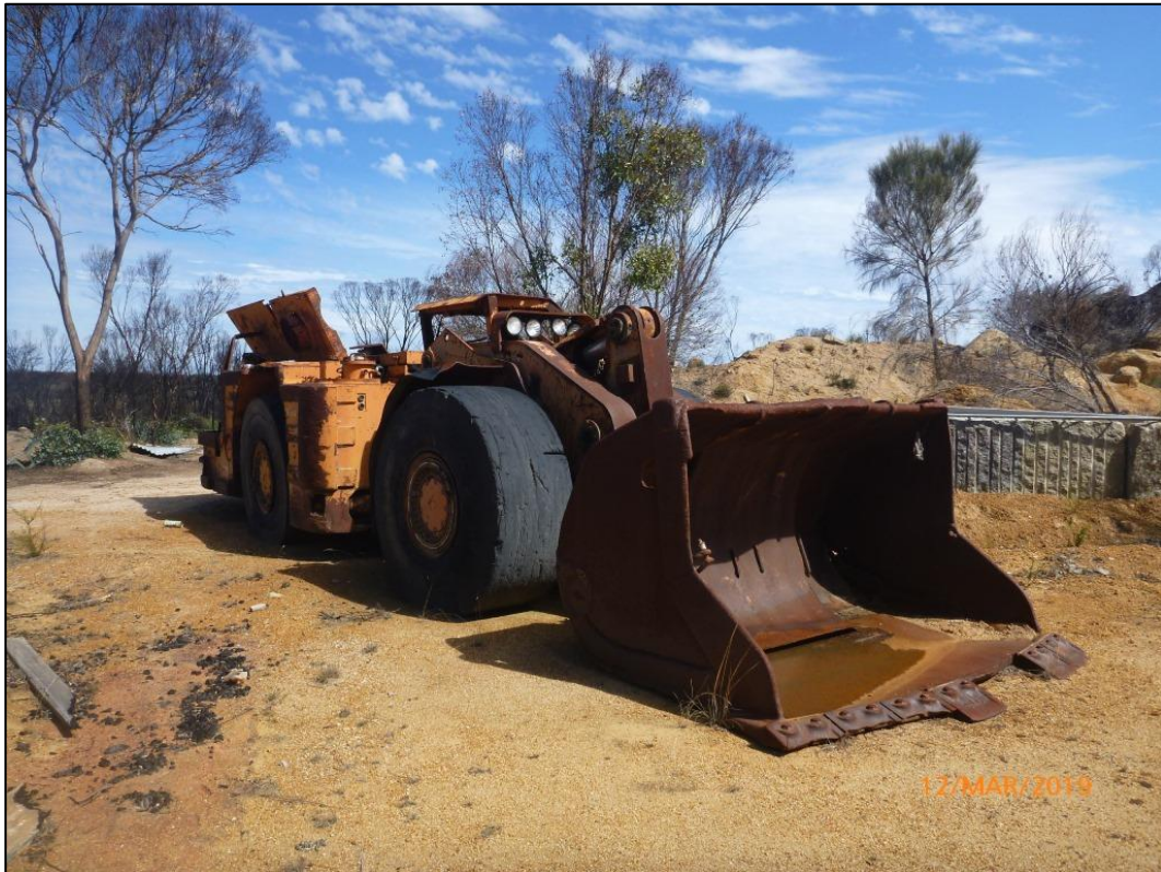
Plate 19: Underground wheel loader “bogger” at workshop area
