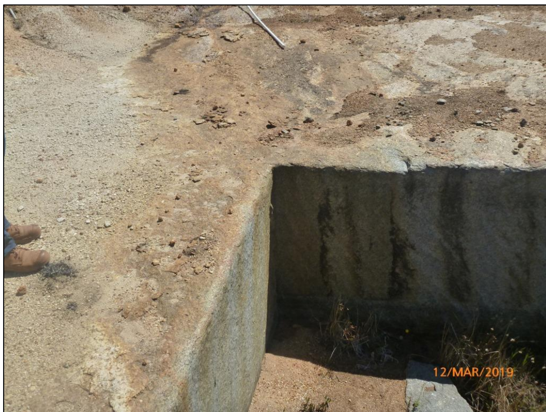
Plate 6: Quarry 1 edges cut with a thermal lance
